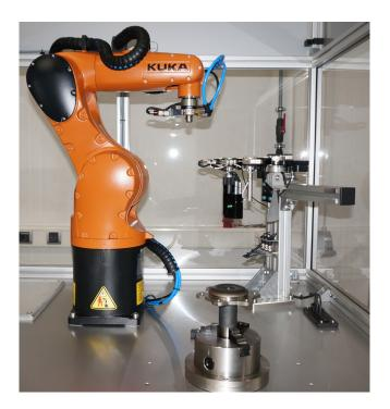
An integrated reference component retainer enables the necessary automatic checking of the system on the basis of reference bodies with defined reference defects. In addition to classic sensors, multiplex sensor arrays or our electromechanical distance compensation EMDC can also be used.
