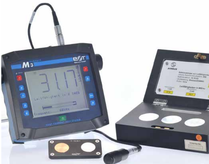
Conductivity measurement in IACS or MS/m from 1 % up to 110% IACS
