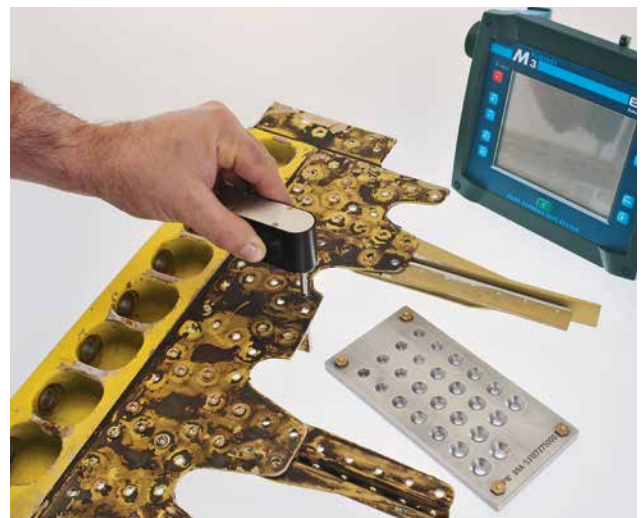
Bore hole inspection with mini rotor on aluminium structures
