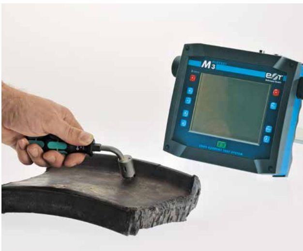
Test set for rough environmental conditions with LED-crack indicator on the probe
